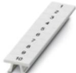
Zack marker strip, white, Printed vertically: consecutive numbers 1 ... 10, 11 ... 20, etc. up to 491 ... 500, mounting type: snap into tall marker groove, for terminal block width: 5.2 mm, lettering field size: 5.15 x 10.5 mm
