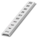
Zack Marker strip, flat, Strip, white, labeled, printed horizontally: consecutive numbers 2 ... 20, 22 ... 40, etc. up to 82 ... 100, mounting type: snap into flat marker groove, for terminal block width: 5 mm, lettering field size: 5.15 x 5.15 mm, Number of individual labels: 10
