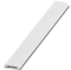
Zack Marker strip, flat, Strip, white, unlabeled, can be labeled with: PLOTMARK, CMS-P1-PLOTTER, mounting type: snap into flat marker groove, for terminal block width: 5 mm, lettering field size: 5.1 x 5.2 mm, Number of individual labels: 10
