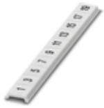
Zack Marker strip, flat, Strip, white, labeled, printed horizontally: Odd numbers 1 - 19, 21 - 39, etc. up to 81 - 99, mounting type: snap into flat marker groove, for terminal block width: 5 mm, lettering field size: 5.15 x 5.15 mm, Number of individual labels: 10
