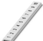
Zack Marker strip, flat, Strip, white, labeled, printed horizontally: consecutive numbers 1 ... 10, 11 ... 20, etc. up to 491 ... 500, mounting type: snap into flat marker groove, for terminal block width: 5 mm, lettering field size: 5.15 x 5.15 mm, Number of individual labels: 10
