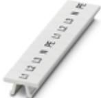
Zack marker strip, Strip, white, labeled, horizontal: L1, L2, L3, N, PE, L1, L2, L3, N, PE, mounting type: snap into tall marker groove, for terminal block width: 5.2 mm, lettering field size: 5.15 x 10.5 mm, Number of individual labels: 10
