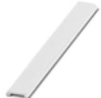
Zack Marker strip, flat, can be ordered: Strip, white, labeled according to customer specifications, mounting type: snap into flat marker groove, for terminal block width: 5 mm, lettering field size: 5.15 x 5.15 mm, Number of individual labels: 10
