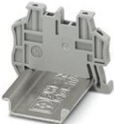
Quick-fit end bracket, inflammability class V0 according to UL 94, for DIN rail NS 35/7,5 or NS 35/15, can be marked with UC-TM 5, UC-TMF 5, KLM 2, KLM3, and KML3L, parking for FBS...5, FBS...6, KSS 5, KSS 6, width: 5.15 mm, color: gray
