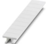
Zack marker strip, can be ordered: Strip, white, labeled according to customer specifications, mounting type: snap into tall marker groove, for terminal block width: 5.2 mm, lettering field size: 5.15 x 10.5 mm, Number of individual labels: 10
